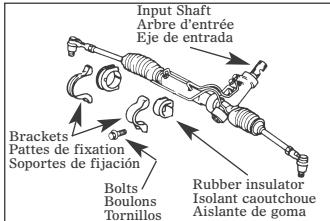
2. Install the mounting brackets, shims, bolts, nuts, washers and insulators in correct position. Torque fasteners to the original vehicle manufacturer's specifications.
