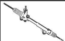
**POWER AND MANUAL RACK AND PINION STEERING**
