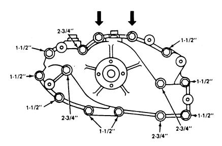
WATER PUMP MOUNTING BOLT LENGTHS & LOCATIONS
