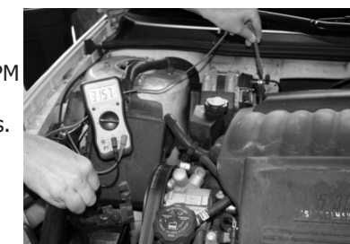
Positive Voltage Drop Test
