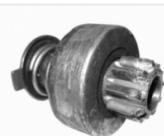
Starter drive damage due to misalignment.
