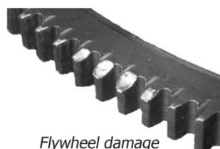
Flywheel damage due to misalignment.
