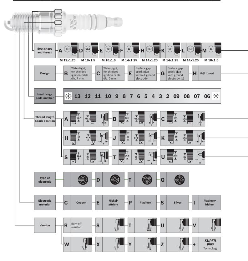
$<sup>^{\</sup>star}$  The thread length for spark plugs with seat shape D and spark position A or B is 10.9 mm.
