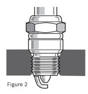
Conical plug installed correctly.
