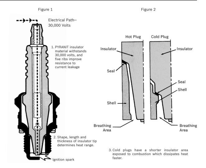
The most apparent difference in spark plug design is variations in thread size, reach and plug height. The plug an engine designer will select depends upon the engine size, performance and operating conditions.
