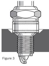
No gasket, danger of pre-ignition. Overheating of the ground electrode, difficulties in removal.
