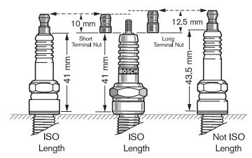
Starting in 1989 Japanese vehicle manufacturers installed spark plugs which conform to ISO standards. The difference in the two plugs can be identified by the letter "K" prior to the heat range number.
