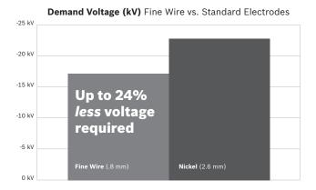
If a non-fine wire plug is used where the OE called for fine wire, demand voltage can be adversely affected leading to weaker spark and lower ignitability. A fine wire plug provides:
