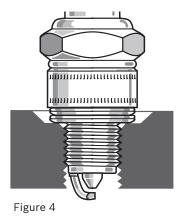
Two gaskets results in cylinder threads becoming filled with residue.
