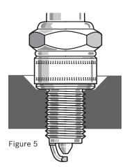
Spark plug with long reach in a cylinder head designed for shorter reach plug.
