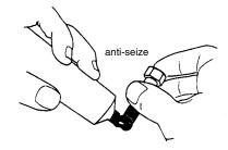
**CLEAN ALL THREADS** by using a wire brush for bolts and studs, tap all bolt holes and stud nuts. Apply a high temperature anti-seize lubricant to the bolt and stud threads.
