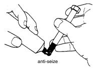
**CLEAN ALL THREADS** by using a wire brush for bolts and/or studs. Apply a high temperature anti-seize lubricant to the bolt and/or stud threads.
