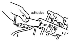
ATTACH AND ALIGN GASKET(S) TO CYLINDER HEAD(S). Apply a quick-drying adhesive sparingly in several places on the cylinder head(s). Mount gasket(s) on cylinder head(s), Allow time for adhesive to set. Test for slippage with light pressure. If gasket moves, allow more time.
