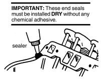
PRIOR TO INSTALLING INTAKE MANIFOLD GAS-KET apply a small dab of silicone sealer to the 4 lower corners where the ends of the block meet with the cylinder heads. **IMMEDIATELY PROCEED** to the next step, as sealer normally sets up in 10-15 minutes.
