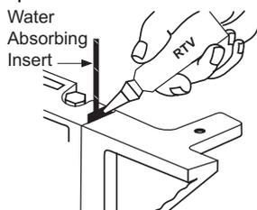
**FILL SIDE SEAL CAVITIES** with silicone sealer (RTV).
