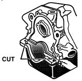
**AFTER REMOVING TIMING COVER, CUT EXPOSED ENDS** of the oil pan gasket flush with the cylinder block using a sharp blade, remove front oil pan end seal.
