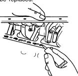
ATTACH AND ALIGN GASKET(S). Apply quick-drying adhesive sparingly in several places on the engine casting or oil pan (depending upon engine model). Mount gasket (or gaskets and seals, if multipiece) on surface where adhesive was applied. Allow time for adhesive to set. Test for slippage with light pressure. If gasket moves allow more time.
