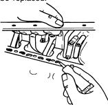
ATTACH AND ALIGN GASKET(S). Apply quick-drying adhesive sparingly in several places on the engine casting or oil pan (depending upon engine model). Mount gasket (or gaskets and seals, if multipiece) on surface where adhesive was applied. Allow time for adhesive to set. Test for slippage with light pressure. If gasket moves allow more time.
