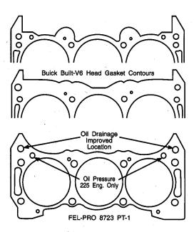
**IMPORTANT:** Buick built V6 engine casting surfaces have different contours for each engine. Avoid intermixing cylinder heads and engine blocks of different displacements.
