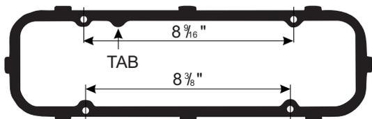
**ATTACH AND ALIGN GASKET.** Apply a quick-drying adhesive sparingly in several places on the mating surface of cover. If gasket has installation tabs, adhesive is **not** required. Mount gasket on cover. **Allow time for adhesive to set.** Test for slippage with light pressure. If gasket moves, allow more time.
