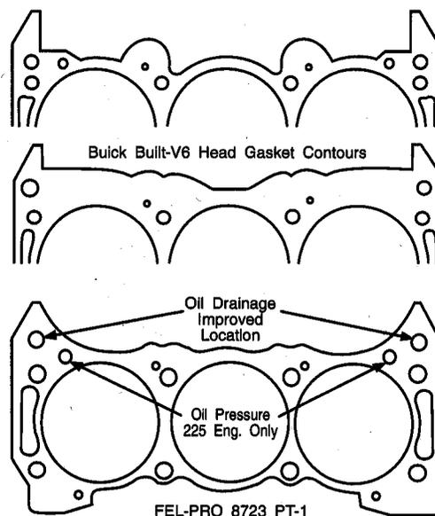
**IMPORTANT:** Buick built V6 engine casting surfaces have different contours for each engine. Avoid intermixing cylinder heads and engine blocks of different displacements.
