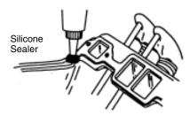
PRIOR TO REINSTALLING INTAKE MANIFOLD apply a small dab of silicone sealer, to the 4 corner intersections between the end seals and gaskets. **IMMEDIATELY PROCEED** to the next step, as RTV normally sets up in 10-15 minutes.
