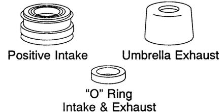
For 1981 and later applications use Positive **Intake** and Umbrella **Exhaust** in addition to the "O" Ring. Prior to 1981 use "O" Ring **Intake & Exhaust** only.
