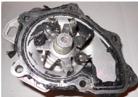
Both pumps were supplied with a rubber / O-ring style gasket. These types of gaskets do not require the use of any sealants.
