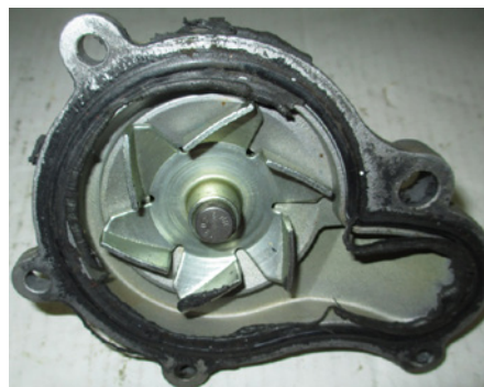
Both pumps were supplied with a rubber / O-ring style gasket. These types of gaskets do not require the use of any sealants.
