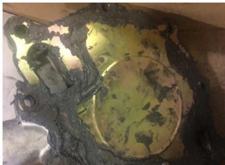
Both pumps were supplied with a rubber / O-ring style gasket. These types of gaskets do not require the use of any sealants.
