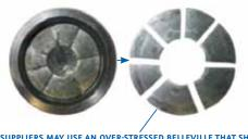
OTHER SUPPLIERS MAY USE AN OVER-STRESSED BELLEVILLE THAT SHATTERS AFTER CYCLIC LOADING, RESULTING IN EXCESSIVE LOOSENESS.
