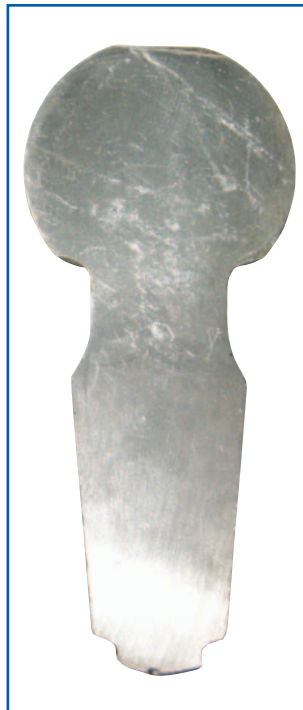
STUD WITH NO INDUCTION HARDENING IS 50% LOWER IN FATIGUE STRENGTH.
