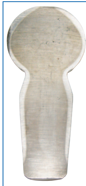
HEAT-TREAT INDUCTION HARDENING CREATES A WEAR RESISTANT SURFACE ON THE BALL AND INCREASES THE FATIGUE STRENGTH OF THE STUD.
