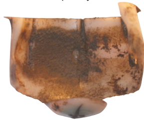
NOTE: Distressed OE style polymer bearing due to rough service conditions.
