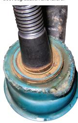
Note: Not all blue-colored boots are created equal. MOOG bellows-style boots (featured on other MOOG applications) are blue in color, but are manufactured from a premium urethane material. These boots will not degrade like blue polychloroprene.
