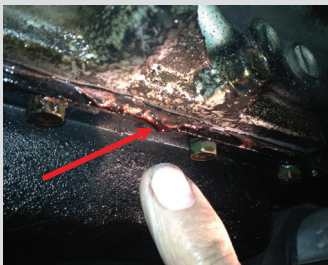
Leak due to gasket not conforming to pan irregularities
