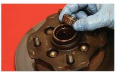
5. Always treat bearings with care. Although bearings appear very durable, they are sensitive enough, that even slight mishandling can damage a bearing's inner geometry.
