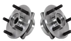
3. PTC recommends replacing the bearings or hubs on both wheels at the same time. Both wheels have the same mileage and are subjected to the same wear and tear.
