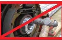
8. Never use a hammer to hit directly on the bearing.
