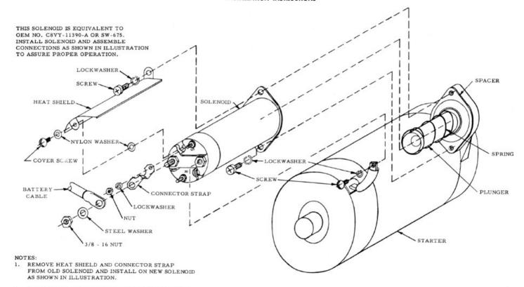
IF THE ORIGINAL SOLENOID HAS THE "R" TERMINAL CONNECTED, RECONNECT SAME WIRE TO "R" TERMINAL ON REPLACEMENT SOLENOID.
