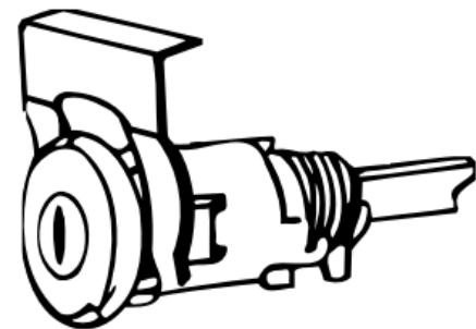
Completely assembled, ready to install. Retainer clip fits up and down as illustrated. Fits on the trunk lid, not on the body.
