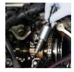
If you're replacing the VVT sprocket, our Master Technicians recommend replacing the VVT solenoid, too. Here are a few repair tips to keep in mind during the replacement:
