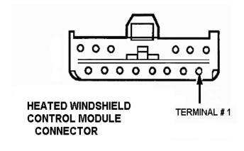
3. Locate the "Alternator Output Control Relay/Heated Windshield Relay" usually found around passenger side inner fender or near battery. Remove the cover. Remove the 16 gauge wire connected to the "M" terminal and tape it back to the harness.
