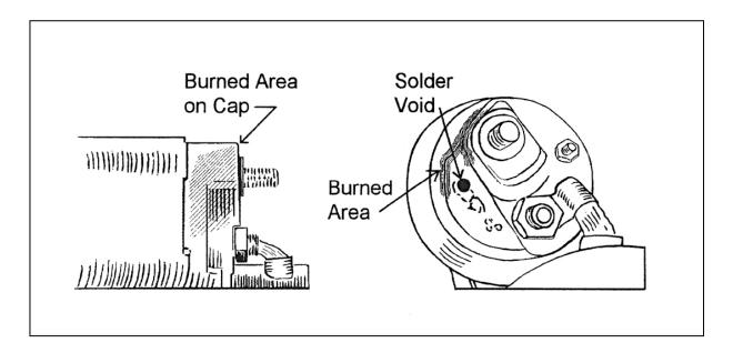
The burned area and melted solder are caused by a defective turbocharger flange gasket. Replace the gasket per OEM recommendations and procedures to prevent reoccurring starter failure.
