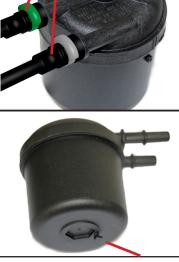
Loosen filter cradle bolt and twist filter slightly to unseat from cradle.
