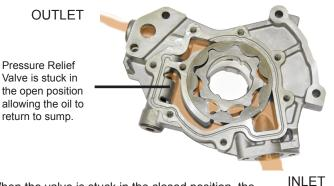
When the valve is stuck in the closed position, the INL lubrication system can be subjected to the maximum flow rate of the oil pump. This equates to an increase in oil pressure.
