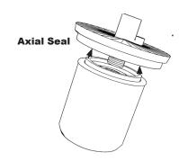
The chemical composition of today's oils and the high operating temperatures of engines are two variables that can affect a gasket over time. More gasket material equates to better chemical resistance to oil and high engine temperatures. This means that the gasket will maintain compression throughout the service life of the filter.
